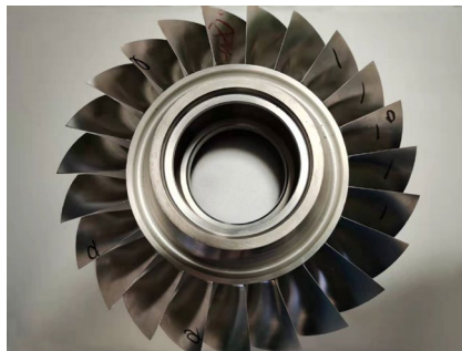
图1 某型号整体叶盘 Fig.1 A certain type of blisk
